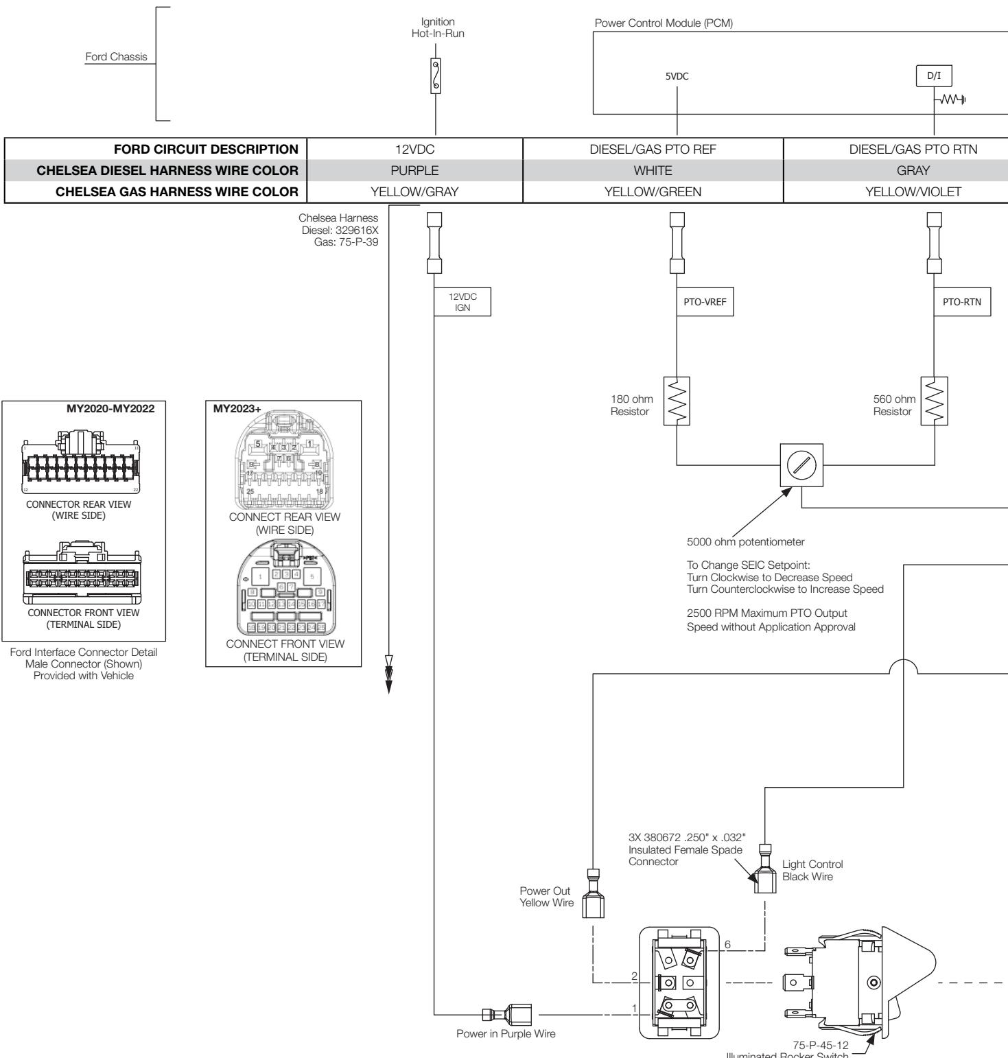
**Wiring Installation PTO to Ford (Cont'd)**
